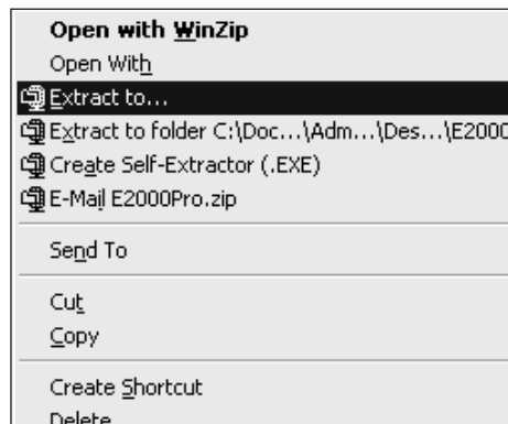
Figure 1-5: Once installed, WinZip allows you to right-click any archive and perform WinZip operations on it
